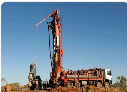
RC drill rig, truck-mounted
